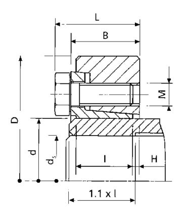
B mm = 85.5 d H8 mm = 180 D mm = 320.0 ds mm = 140 F kN torque = 1157 H = 8.0 I mm = 71.5
